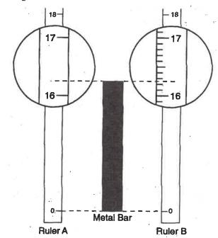
What is the greatest degree of precision to which the metal bar can be measured by ruler A and by ruler B?
