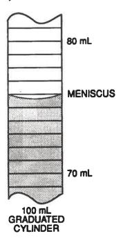
When the meniscus is read to the correct number of significant figures, the volume of water in the cylinder would be recorded as
